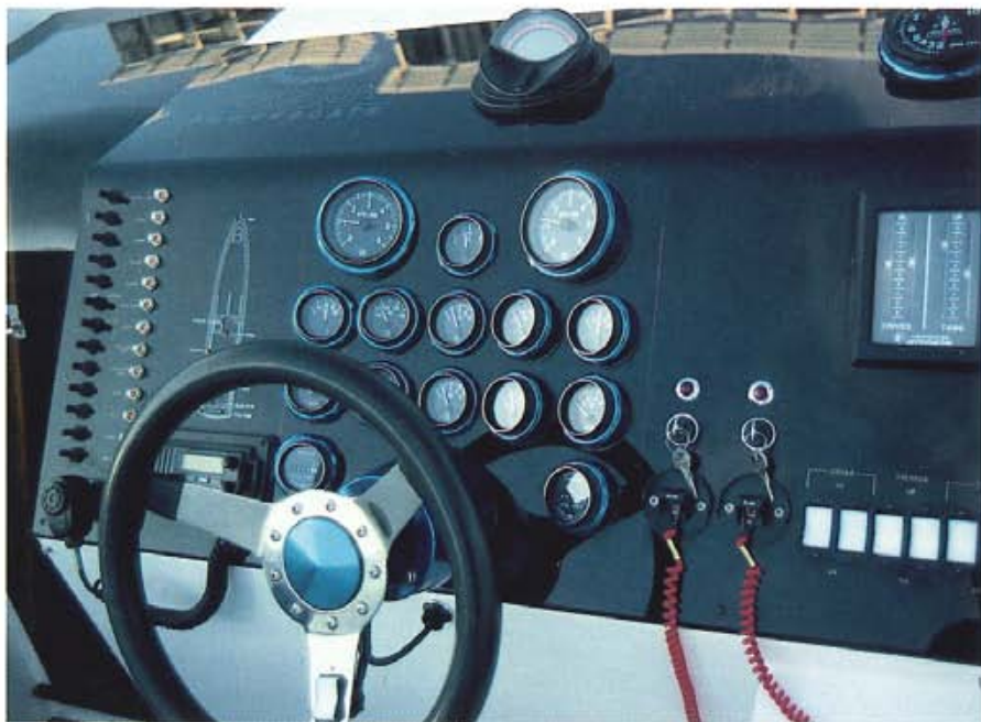
The 37's dash featured a digital compass and a pictograph to identify accessories.
