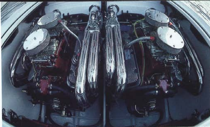
Innovation mills, Holley rams, Stelling's exhaust, and Gil strainers made the 37 sing.
