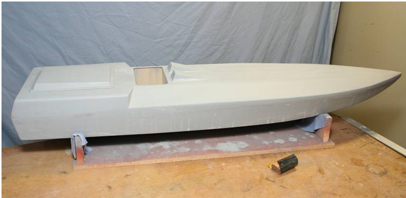
A couple coats of grey primer-surfacer, wet sanded. Note the hatch and instrument "pods" in place.
