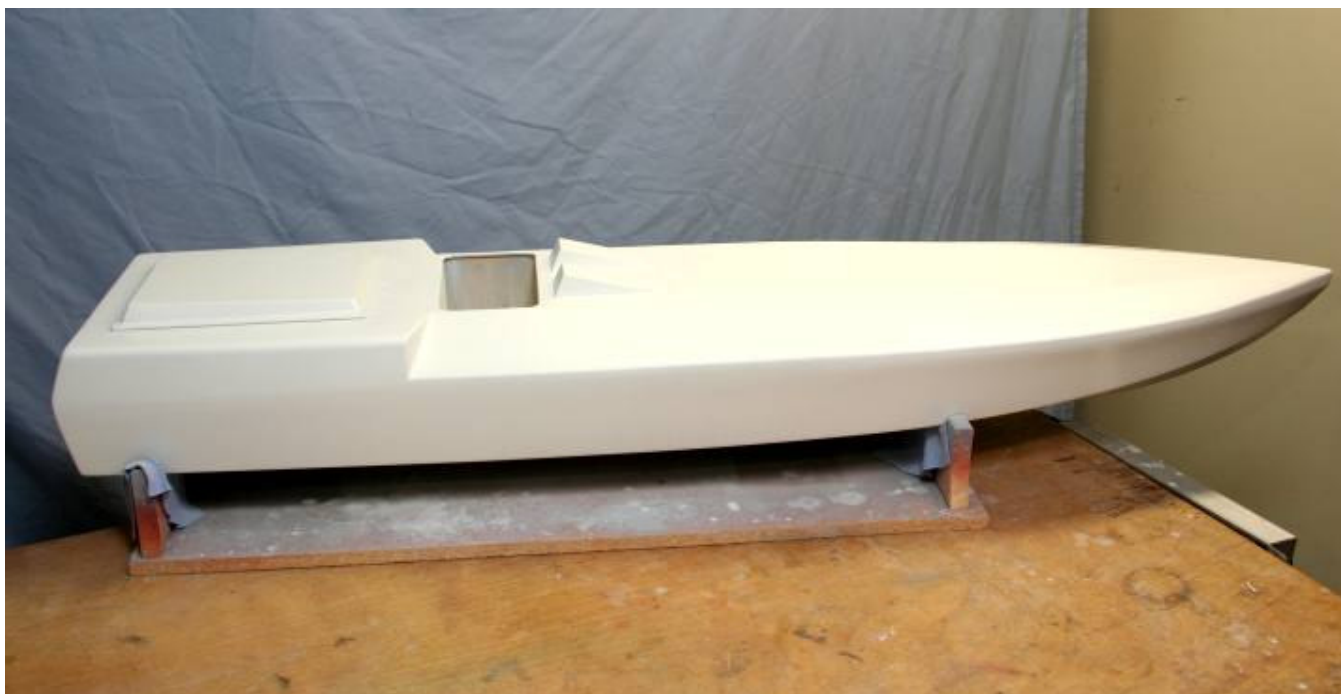
And now it's white! Lacquer, in the middle of being rubbed out. Next, mask and paint the red.
