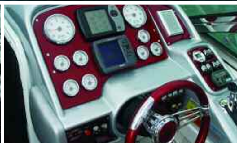
Mercury Racing's HP700SCi's provide the 382's punch. A red carbon-fiber dash panel flaunts Livorsi instrumentation, a Garmin GPS and Mercury's SmartCraft SystemView.
